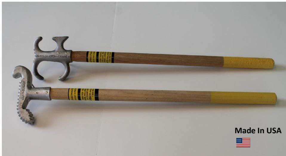
Greatly minimize the risk of serious hand injuries with the Alpenco Saf-T-Guider™. The Push/Pull, lightweight tool is used for the hands-free guiding and directing of heavy crane and fork lift loads. Made with an Ash Hard Wood pole with a serrated cast Aluminum head for ease of arm extension during long reaches. The 18" and 24" models can be carried on your tool belt for quick access and weighs under 2 lbs. **Sizes:** 18", 24", 36", 48", 72", 96", and 120"(special order)
